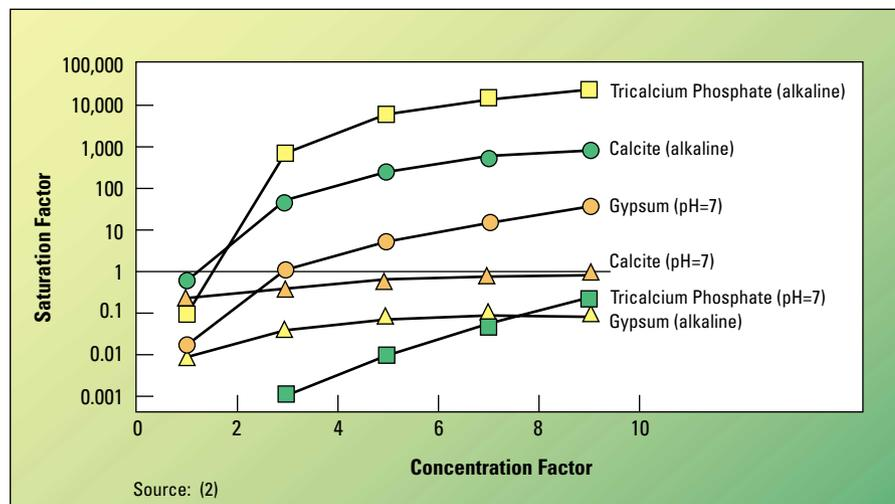
Figure 3. Impact of cycling on saturation factors of scalants. Source: (2).
