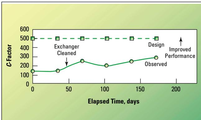
■ Figure 5. Diagnostic study of heat exchanger  $C$ -factors with fluorescent inert tracers.
