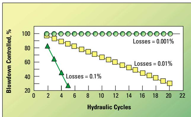
Figure 1. Total water losses under blowdown valve control.
