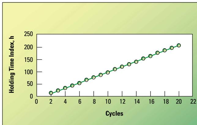
Figure 2. Increased cycling increases the holding time index.
