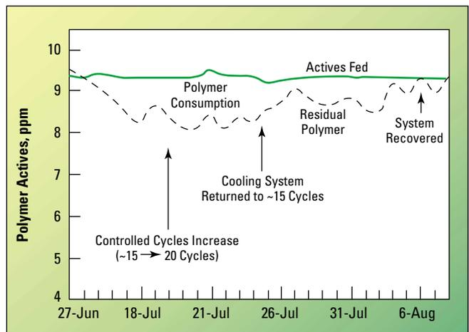
■ Figure 8. Effect of increased then decreased cycles of concentration on dispersant polymer consumption.
