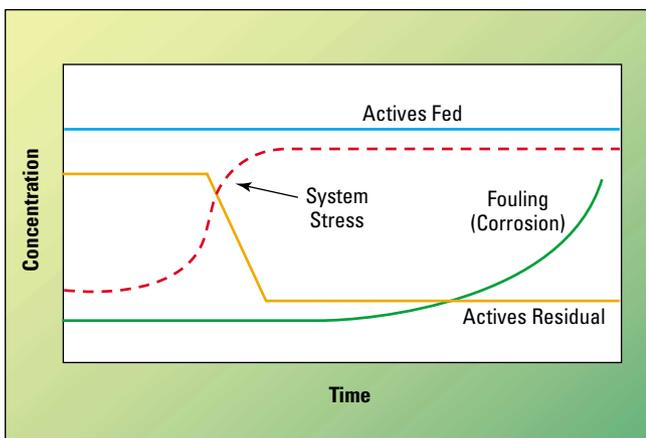
■ Figure 6. Effect of increased system stress on treatment dosage, actives consumption, and performance.
