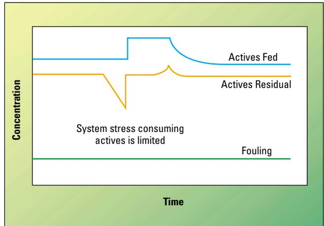
■ Figure 7. Treatment dosage and actives consumption measurements to automatically respond to system stresses.
