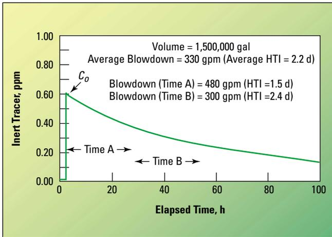
■ Figure 4. Diagnostic tracer study of total system volume and blowdown rate.
