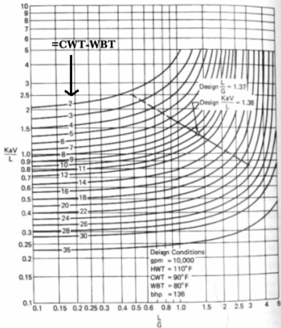
Figure 7: A Typical Set of Tower Characteristic Curves
