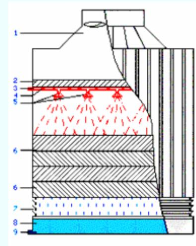
1. Fan; 2. Drift eliminator; 3. Warm water; 4. Water distribution; 5. Water sprinkling nozzle; 6. Fill packing; 7. Air inlet; 8. Water pool; 9. Cooled water
