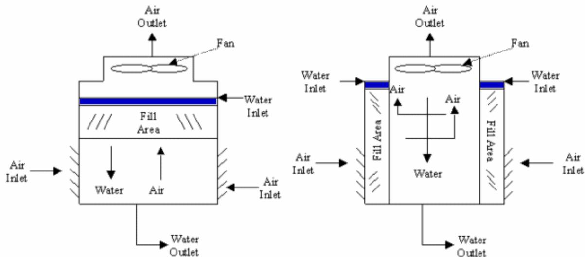
*Figure 2: Mechanical Draft Counterflow Tower*
