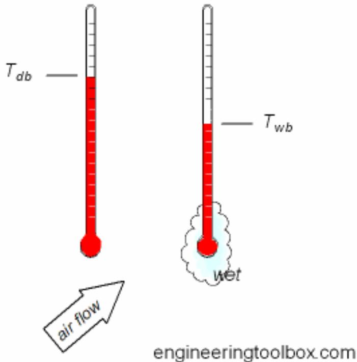
Temperature can be measured with two thermometers simultaneously - one with a wet bulb and one with a dry bulb- in order to determine the relative humidity of the surrounding air. This method was used historically by meteorologists, but we will use it extensively in this experiment to measure the water concentration in the air.
